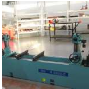
ROBBI R 2000-C Machining coaxial holes 22-200 mm and up to 2200 mm long, machining accuracy 0.01mm
