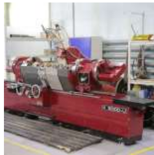
AMC Schou K2000U Machining of the engine crankshafts
