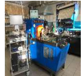
Stand CDT - 22 Diagnostics of fuel pumps and high pressure injectors and common rail systems
