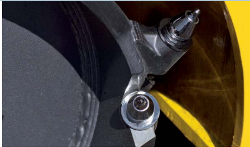
The special geometry of the edge cutter gives a smooth edge. Diagonal cutters protect the rotor around bends.
