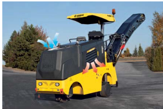
Sound insulation and intelligent air duct.
