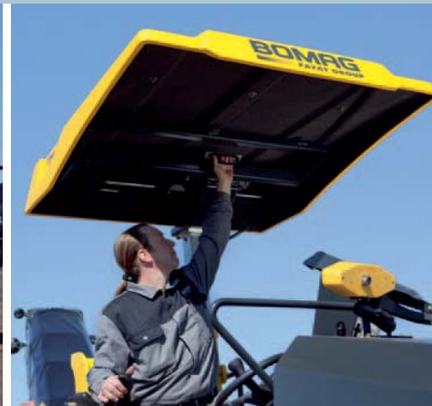
And the roof can be easily shifted laterally, ideal for confined site conditions.
