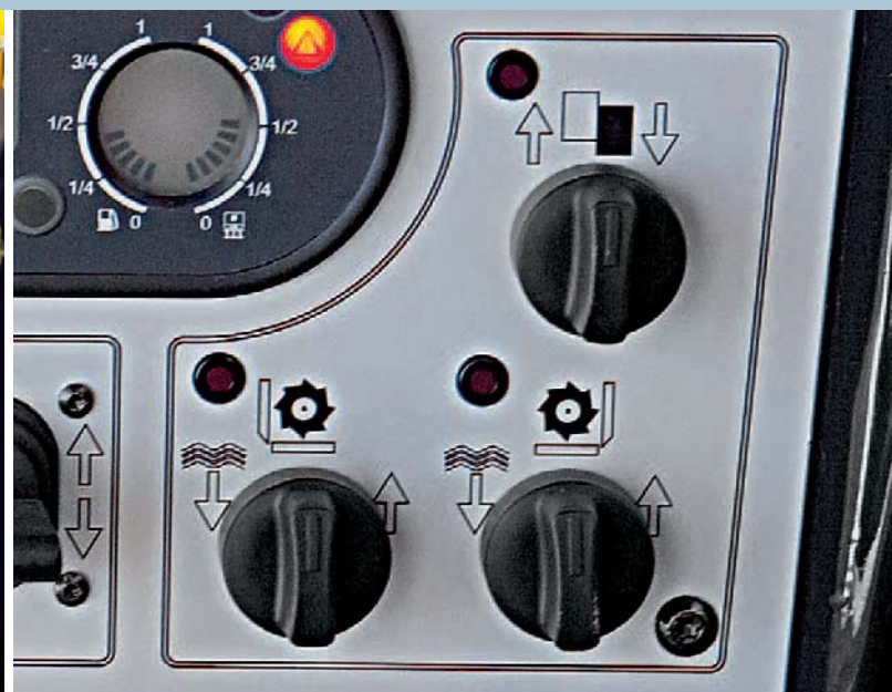
The split design scraper door can also be controlled from the panel.
