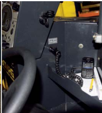
24 V sockets for headlights and 12 V connections for the cool bag.
