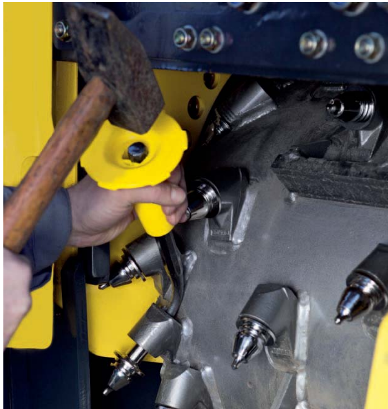
Ultimate easy access for servicing and simple, fast knocking out of cutters from the rear speeds up maintenance.
