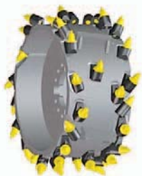
Quick-change Milling Drum
