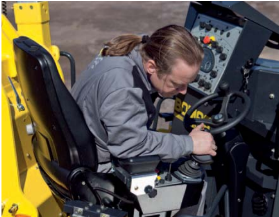
The 45 degree swivel seat which gives a clear view to the loading truck and edge.
