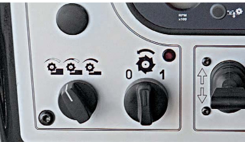
Manually adjustable – the best cutting speed for any application.
