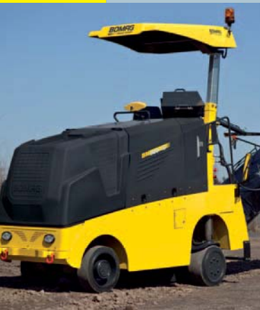
The large, optional weather protection roof is height adjusted from the seated position with no interruption to work.
