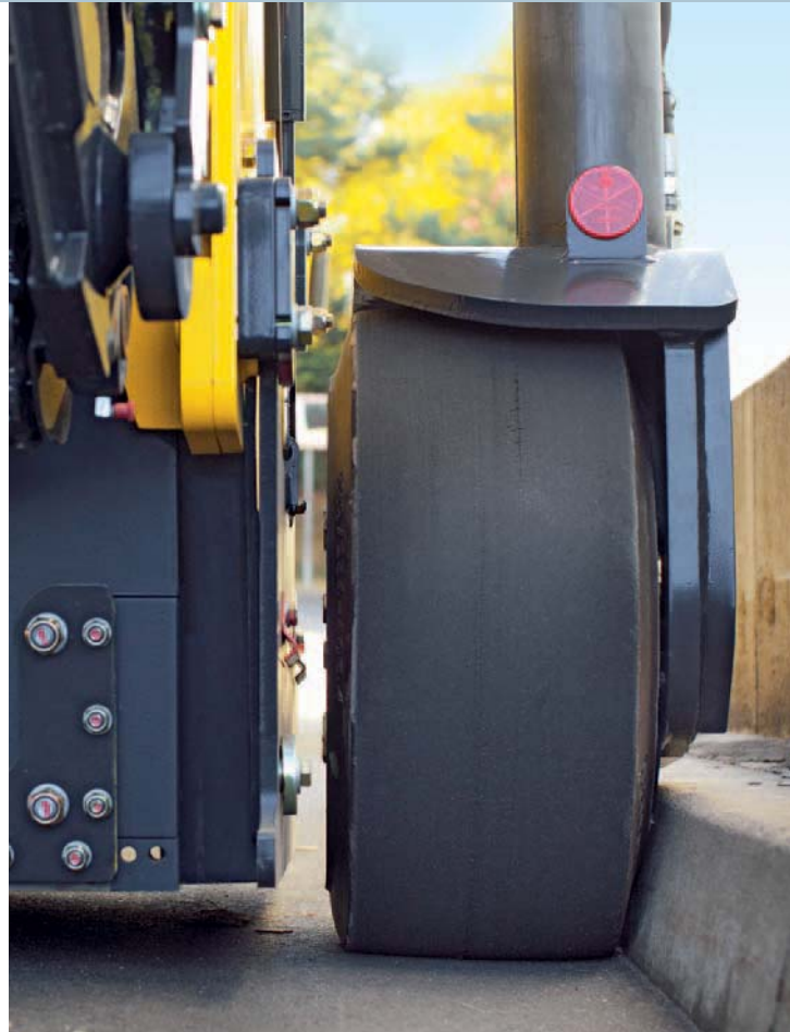
Extra ground clearance with optimised gear housing.
