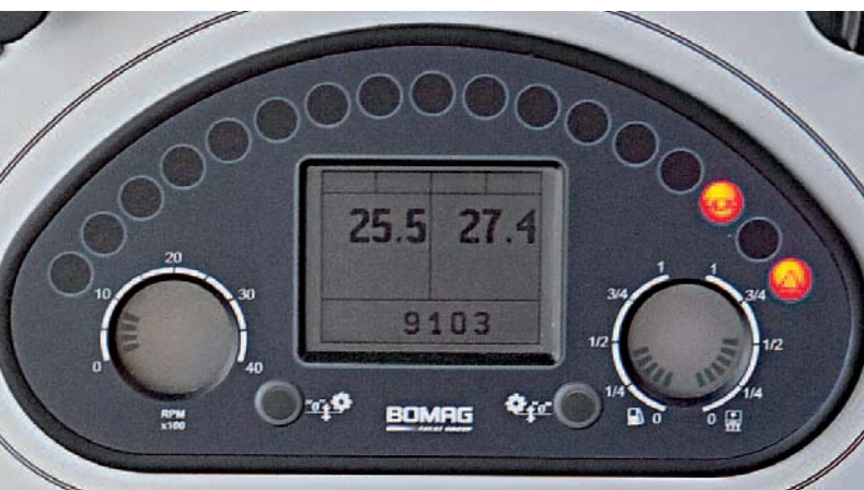
The digital milling depth display and the switch for the travel speed are in the operator's direct line of vision.
