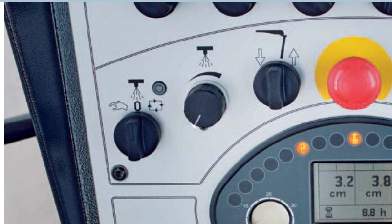
Spraying can be controlled easily using two control switches.
