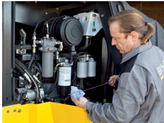
All maintenance points are easily accessed through the wide opening engine hood on one side.
