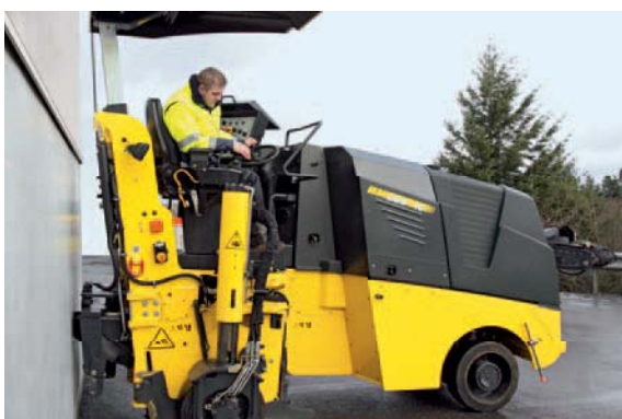
No control cylinder to affect the rear of the planer.
