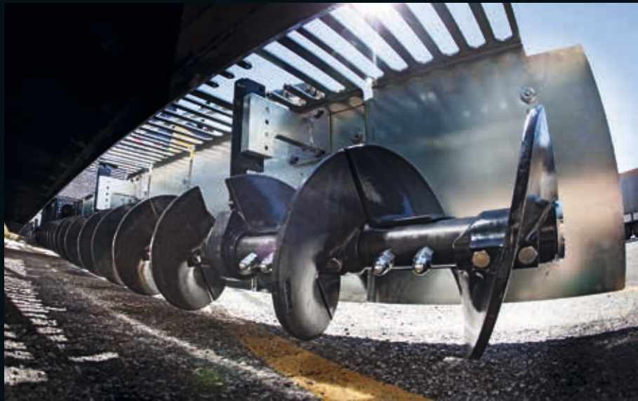
Optimal material distribution: the generously dimensioned auger diameter.
