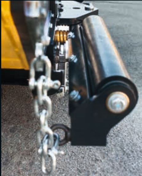
Impact-free docking thanks to 22 dampened bumper rollers.
